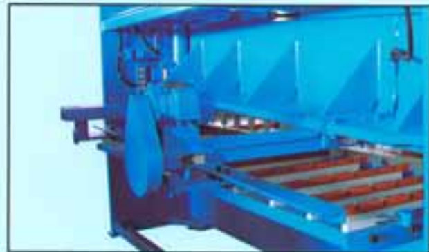
B) Sheet Support-Up position. Ready for the next cut.
